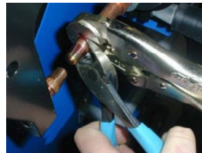
Figure 5.6b: Removing Welding Cap
