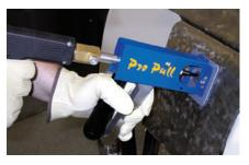
Position the weld tip on the bottom of the dent, weld, then squeeze the handle of the Pro Pull to initialize the pulling action.
