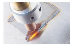
Ideal for rust repair and patching, stitch welding works by delivering an intermittent or pulsating current while rolling the tip on the sheet metal edge.
