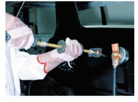
Quickest dent pulling system ever! Just weld the Spot Hammer directly on the dent and hammer away pulling the dent. Simply twist to release (magnetic ground plate optional).
