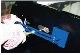
Simply weld on the shaft to the dent and use the Lever Bar to pull and straighten out dents.
